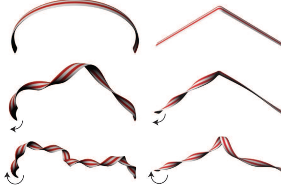
Figure 4.2: Anisotropy of the cross-sections and natural curvature of the centerline “conspire” to produce non-uniform twist distribution. From top to bottom: reference configuration, moderate twist, large twist.
