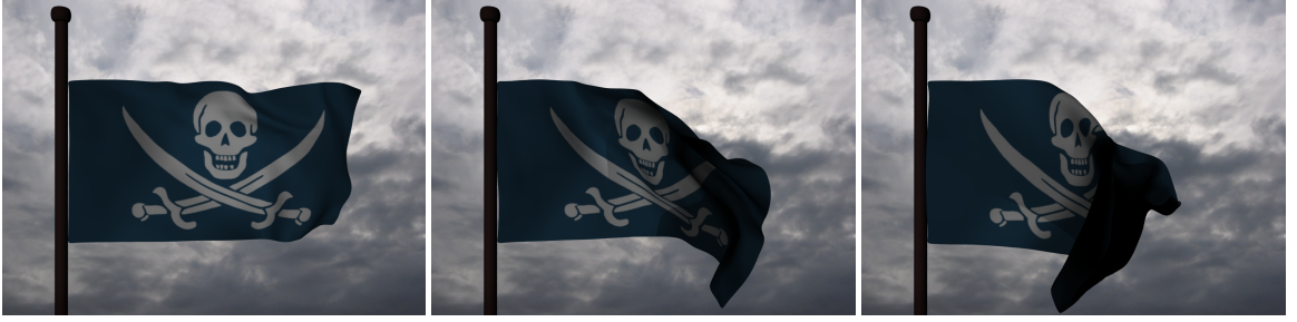
Figure 2.1: These images show snapshots from a simulation of a flag using the isometric bending model to compute bending forces. Despite its economy of cost, the proposed bending model achieves qualitatively the same dynamics as popular nonlinear models.
